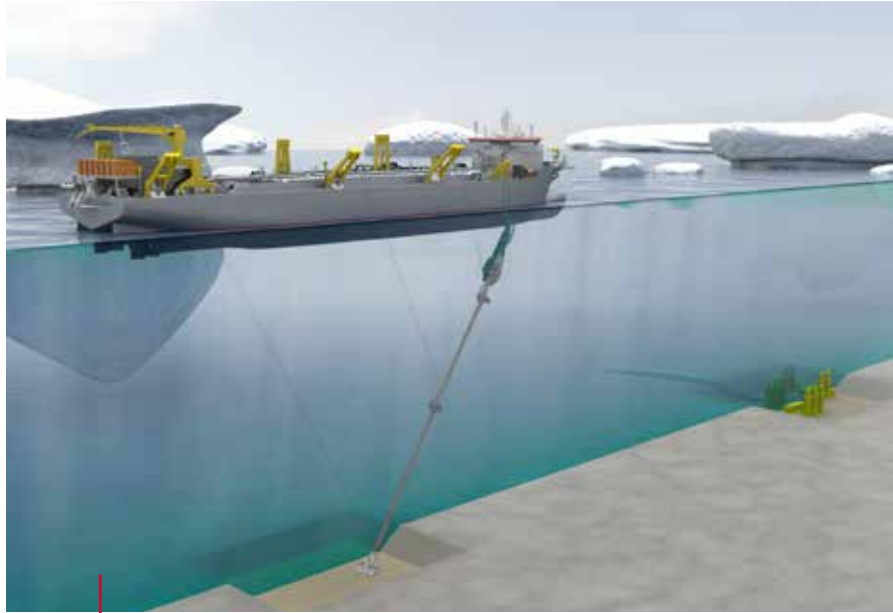
The trailing suction hopper dredger Cristóbal Colón dredges excavations on the seabed of the Atlantic Ocean for the installation of production pits along which gas or oil will be won.
