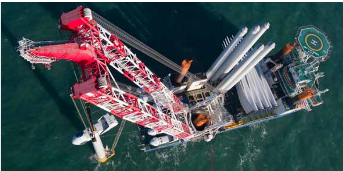
The offshore installation vessel Vole au vent installs wind turbines at sea.
