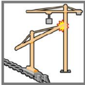
Jib of travelling crane hits mast of interfering crane, or other obstacle
