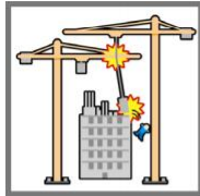
Hoist rope of high crane, hit by jib of low crane – the load is jolted and the banksman thrown off balance
