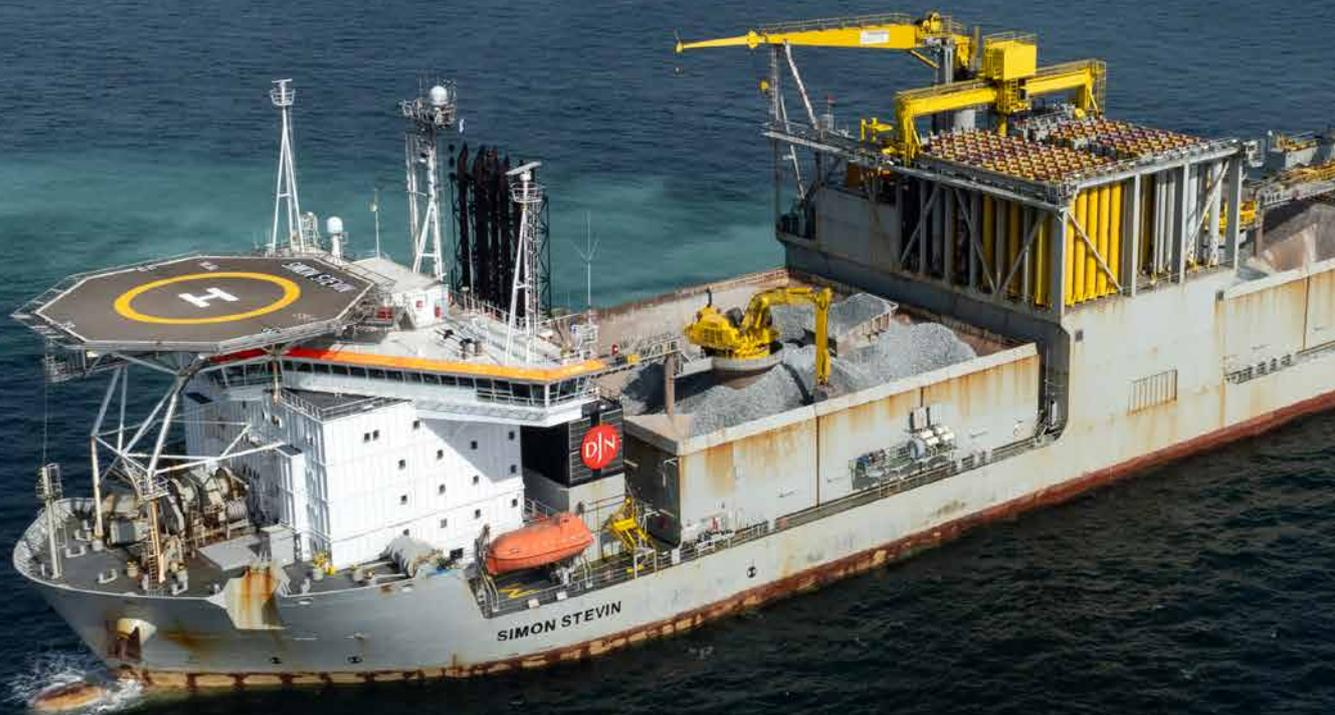
In the Belgian North Sea, we are building the Princess Elisabeth Island, the world's first artificial energy island. Twenty-three armoured concrete blocks will form the contours of the island. To create a firm foundation for the caissons, our rock installation vessel Simon Stevin placed rocks on the seabed.
