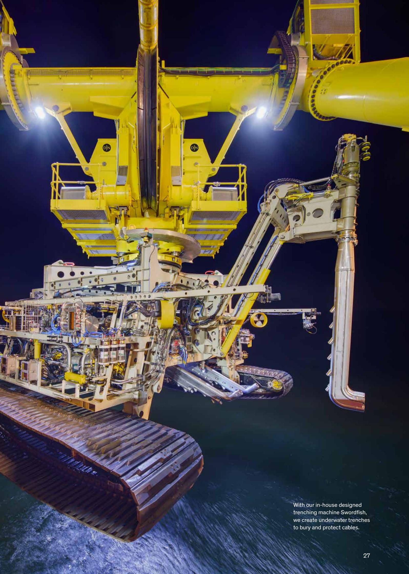
With our in-house designed trenching machine Swordfish, we create underwater trenches to bury and protect cables.
