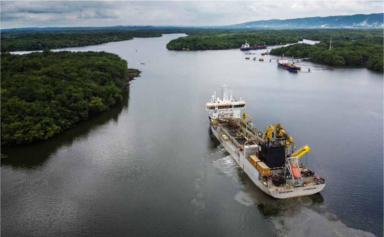
To keep the port of Guayaquil, Ecuador, accessible to Neo Panamax and other large vessel sizes, we deepened its access channel to 12.5 metres.
