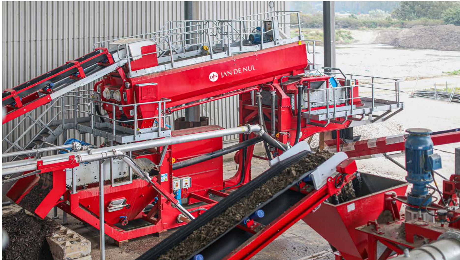
In 2023, we commissioned our third PFAS washing plant in Ghent, in addition to our plants in Liège and Toulon in France. Together, the three plants can make up to 2,000 tonnes of soil PFAS-free every day.
