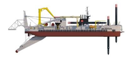
138.5 m Length o.a. Breadth 26 m 5.5 m Draught 35 m Dredging depth 900 mm Suction pipe diameter 900 mm Discharge pipe diameter Barge loading pipe diameter 900 mm 4,250 kW Submerged pump power Inboard pump power 2 x 5,000 kW Cutter power 7,000 kW 2 x 3,500 kW Propulsion power 23,520 kW
