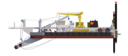
Length o.a.86.7 mBreadth19 mDraught2.95 mDredging depth20.5 mSuction pipe diameter900 mmDischarge pipe diameter800 mm
