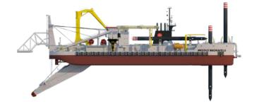
138.5 m Length o.a. Breadth 26 m 5.5 m Draught 35 m Dredging depth 900 mm Suction pipe diameter 900 mm Discharge pipe diameter Barge loading pipe diameter 900 mm 4,250 kW Submerged pump power 2 x 5,000 kW Inboard pump power Cutter power 7,000 kW 2 x 3,500 kW Propulsion power 23,520 kW Total installed diesel power
