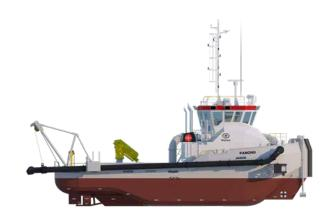
Length o.a. 30.33 m 10 m Breadth moulded Breadth o.a. 13.2 m Max. draught 3 m Bow thruster power 150 kW 735 kW Jet water pumps 10,000 m<sup>3</sup>/hr Flow rate pumps 12.35 m Width sweep beam 2 x 735 kw Propulsion power Total installed diesel power 2,376 kW Speed 10 kn 6 Accommodation 2021 Built in / Converted
